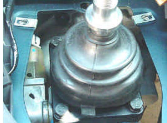
*(I installed the factory dust cover back on the MGW shifter. The directions omitted this step, as it is not necessary.)*
