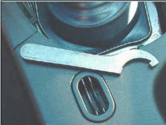
*(You will need to use this special tool called a Spanner wrench to tighten the shifter's locking nut)*
